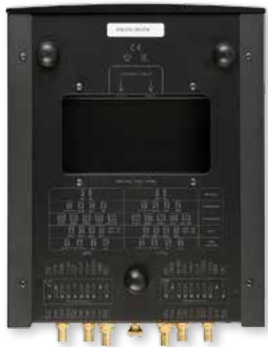
ABOVE: The DIP switch permutations for input, loading, gain and subsonic filtering are illustrated under the case, beneath a void for the dual PSU inputs
