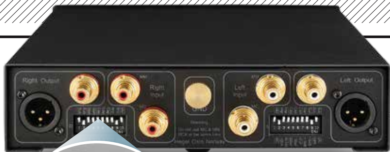
ABOVE: Separate RCAs are provided for MM/MC inputs, selected via a DIP switch, alongside other toggles for gain, loading and subsonic filtering – see detail [inset]. RIAA eq'd outputs are offered on RCAs and balanced XLRs
