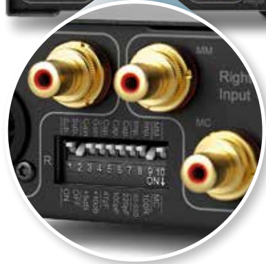
ABOVE: Separate RCAs are provided for MM/MC inputs, selected via a DIP switch, alongside other toggles for gain, loading and subsonic filtering – see detail [inset]. RIAA eq'd outputs are offered on RCAs and balanced XLRs
