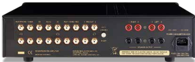
ABOVE: The 3510 offers five line inputs (one for an MM/MC phono option), a tape loop and two preamp outs. Dual 4mm speaker cable sockets support bi-wiring but are for banana plugs only – no bare wire or spade lugs here!
