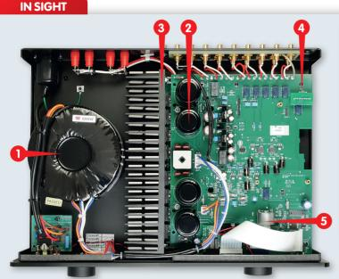
Substantial toroidal mains transformer feeds...
