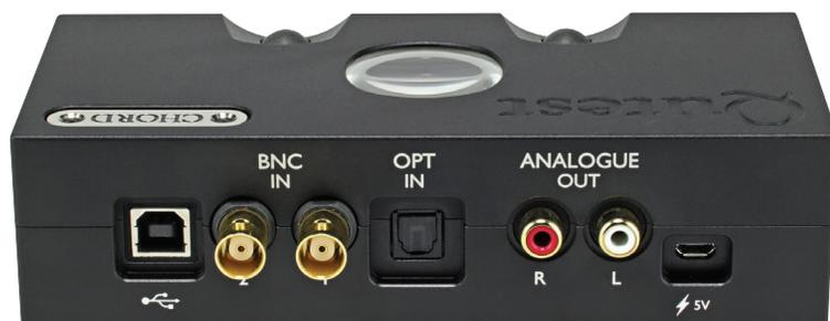
**Digital input (S/PDIF) is via gold plated BNC connectors, rather than the usual RCA phono sockets, so BNC terminated connecting leads are required. Otherwise socketry is conventional, except that the micro-USB socket at right is a power input only.**
