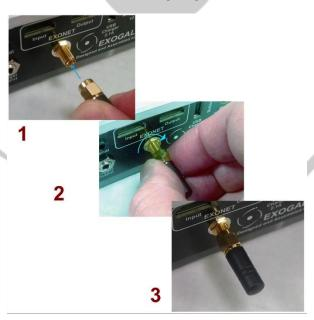
Simply screw the antenna onto the matching RF connector on the back of the Comet.
