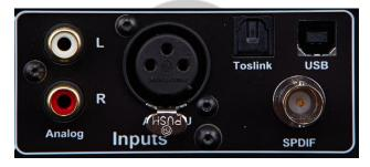
To connect a source, install the proper cable between the output of that source and the matching input of the EXOGAL Comet.
